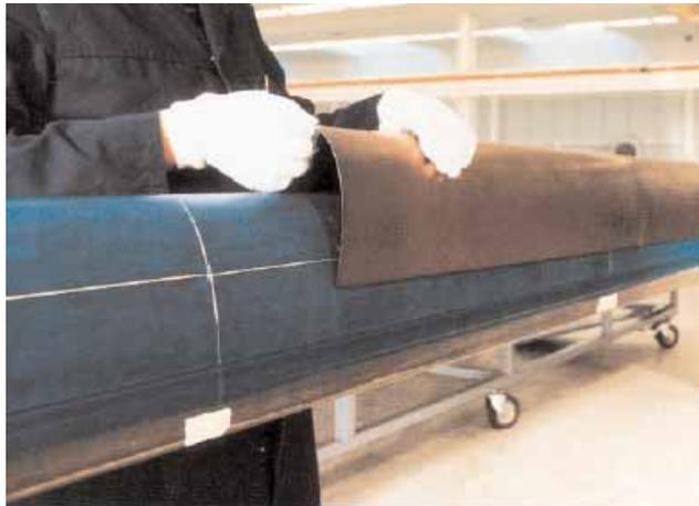
*Helicopter leading edge – The first 250°F (121°C) curing film with a 300°F (149°C) service temperature, AF 3109-2 bonds titanium leading edge to the de-icer mat in spar assembly. Co-cured with prepregs at 250°F (121°C), AF 3109-2 goes through secondary cure cycles without stress to the structure.*
