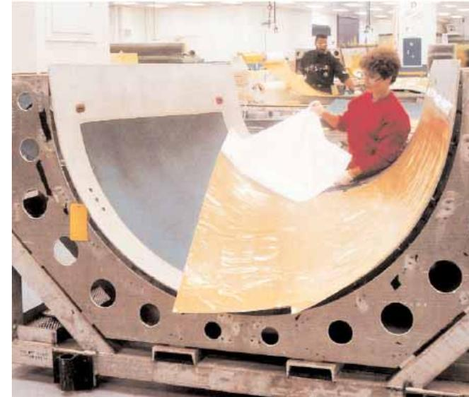
*Nacelle assembly – With 1700 psi overlap shear at 300°F (149°C) and 40 piw T-peel, AF 30 Adhesive Film bonds the aluminum skins of engine nacelles — an application demanding resistance to sonic fatigue.*
