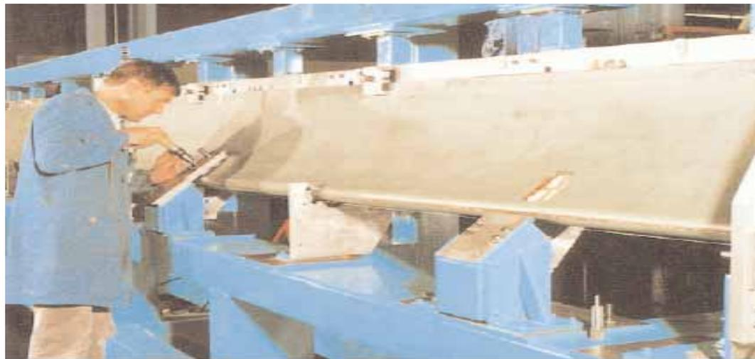
*Commercial transport flap vane – AF 163-2 bonds the skin to the core in assembly of a flap vane, shown here in fixture after autoclaving.*
